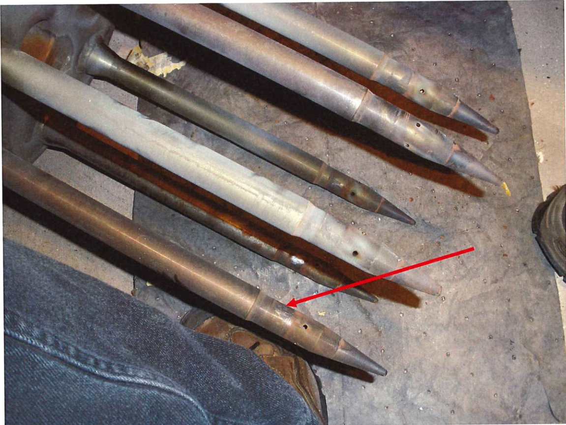
Main fuel nozzle from burner #8. Note some minor signs of fretting at the base of the tip where it goes through the swirler guide.
