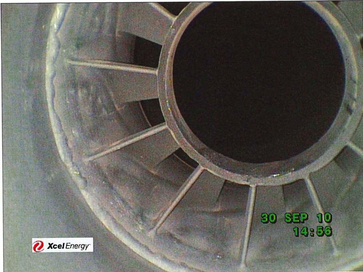
Pilot swirler on burner 14 indicates some minor fretting in the guide tube, but again nothing serious.
