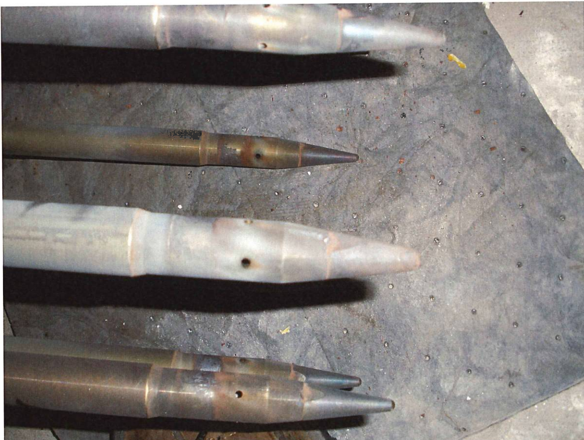
Closer view of the rocket nozzle tips on the main fuel nozzle from burner #8. Note the relatively blunt tip on one of the rockets (close-up in next photo).
