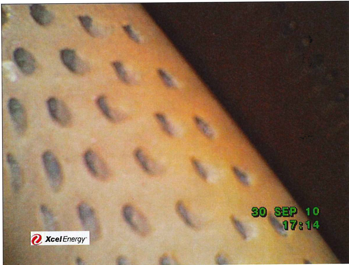
Close-up view of the row 1 vanes at #8 burner. Once again no obvious signs of damage or distress.
