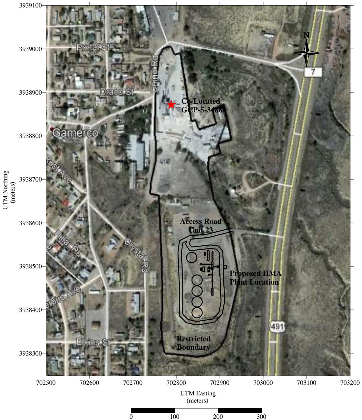
Figure 5-1: HMA Plant Site Layout
