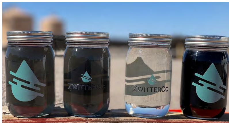
Figure 5: Picture of the raw produced water, SF feed (cartridge filtered produced water), permeate, and concentrate from left to right.
