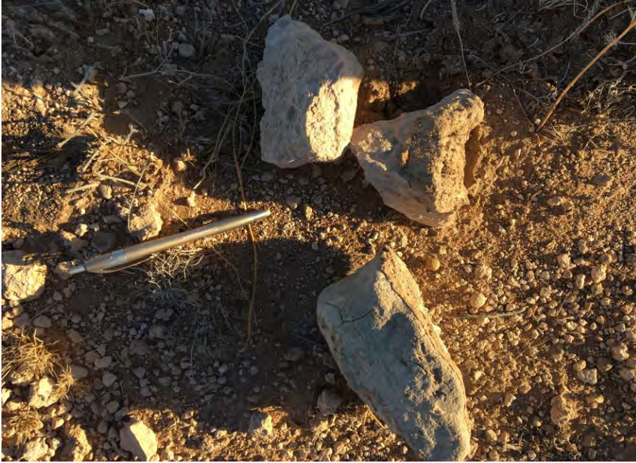
Figure SP-7 Close up showing nature of alluvial deposit with sub-rounded dolomite cobbles, within a matrix of smaller rounded clasts and some angular clasts.
