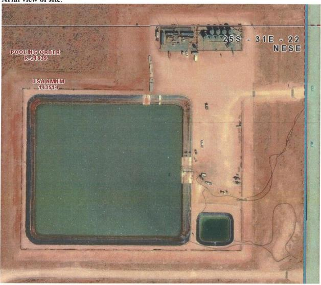
• **Produced Water Source and Quality**: (produced water source and general quality in ppm TDS). The produced water source is from the Wolfcamp, Bone Spring and Avalon formations around the treatment facilities. The TDS of the water is generally between 115,000ppm and 130,000ppm.
