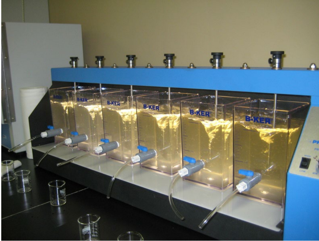
Figure 1. Phipps & Bird jar testing apparatus with B-KER2 jars.
