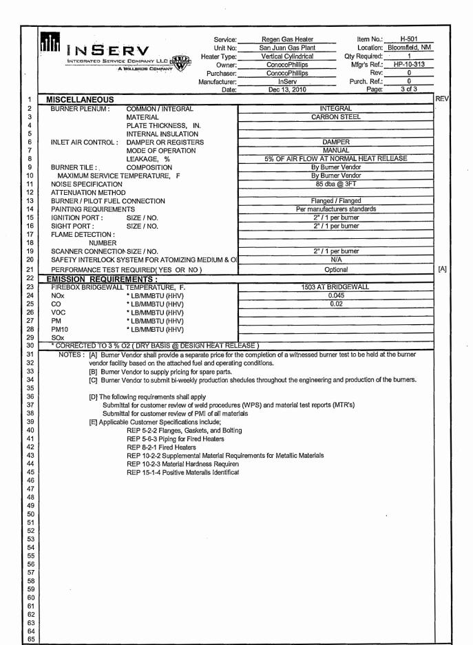
InServ Burner Data Sheet API Standard 560
