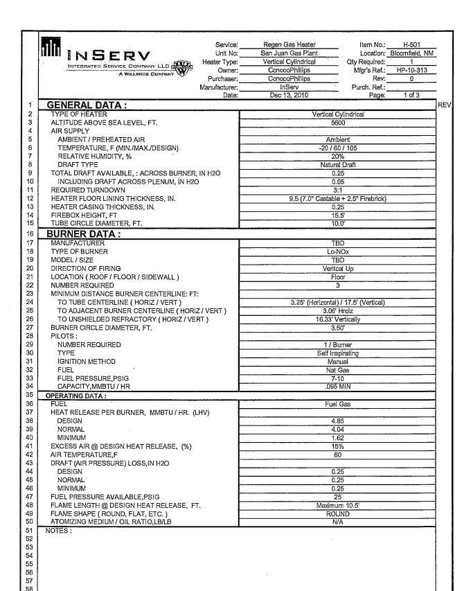
InServ Burner Data Sheet API Standard 560
