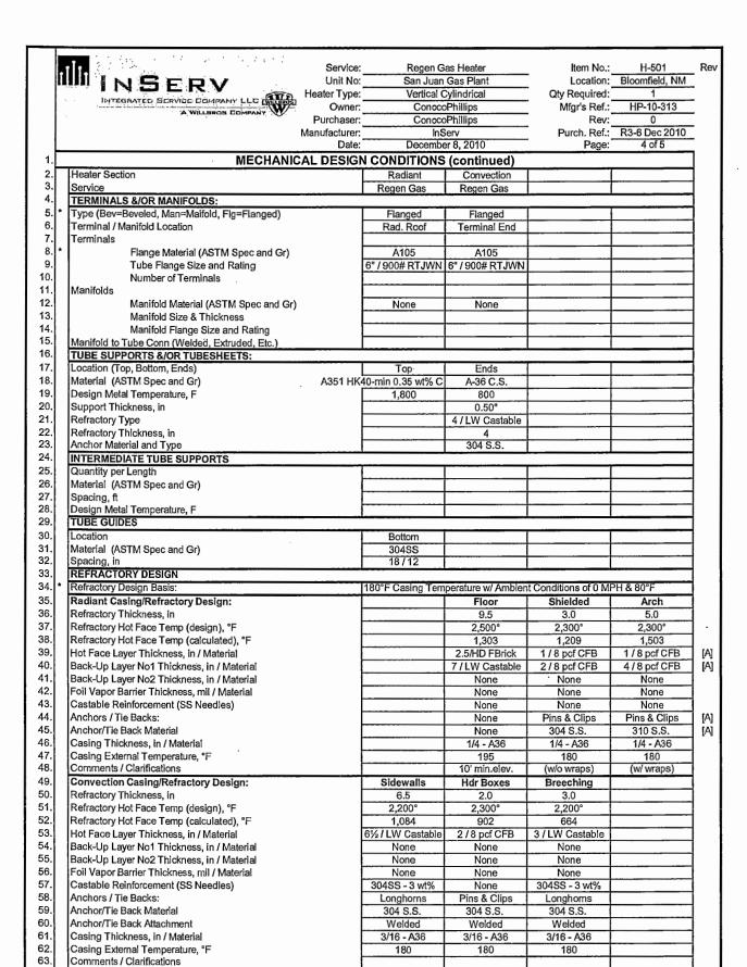
[A] Floor refractory and firebrick will be field installed and therefore no anchors are required per API 560.
