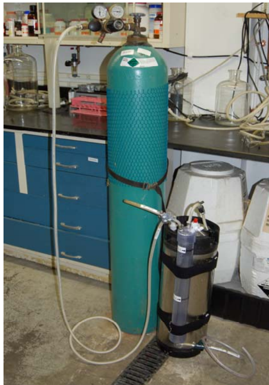
Keg and measuring cylinder connected to delivery gas tank.
