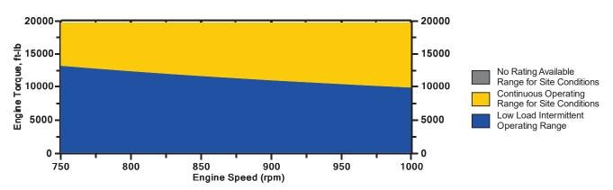
Note: At site conditions of 500 ft and 77°F inlet air temp., constant torque can be maintained down to 750 rpm. The minimum speed for loading at these conditions is 750 rpm.
