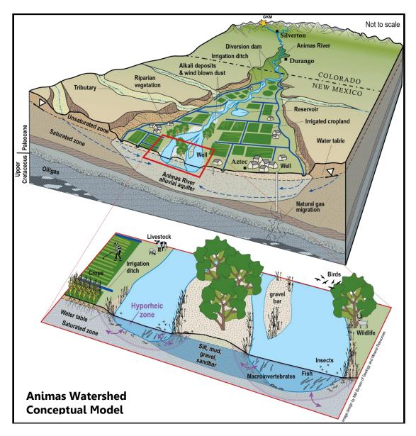
Conceptual Illustration of the Animas River Hydrologic System. Many of the potential pathways for contaminant migration addressed by the Long-Term Monitoring Plan are identified on this image. Image courtesy of NM Bureau of Geology and Mineral Resources, developed with feedback from the Long-Term Impact Team.
