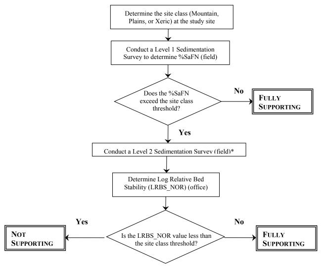
Figure 2. Generalized flowchart for determining sedimentation/siltation impairment
