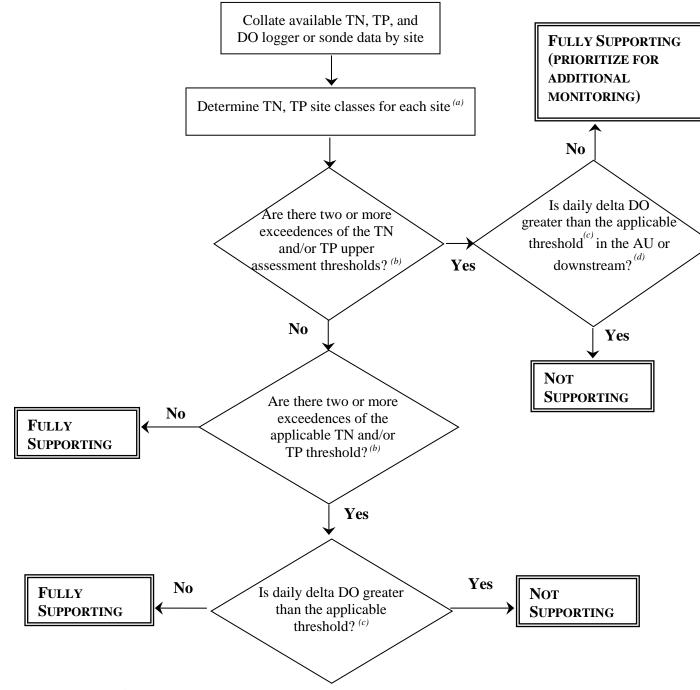
Figure 4. Generalized flowchart for determining nutrient impairment
