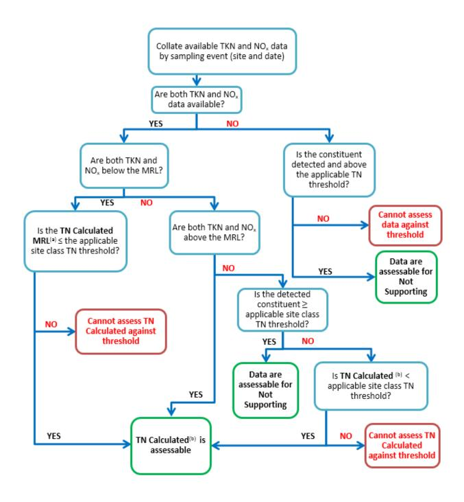
Figure 3. Generalized flowchart for calculating and determining TN Calculated data usability
