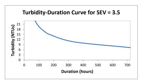
**Figure 1**. Relationship between turbidity and length of exposure for a SEV index of 3.5 with respect to New Mexico's narrative turbidity criterion, based on Newcombe (2003)
