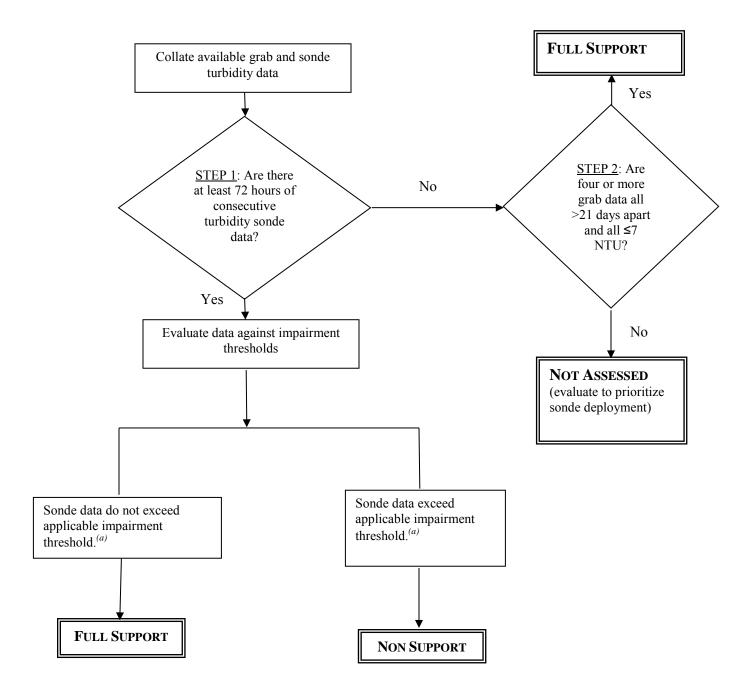
**Figure 1.** Generalized flowchart for determining turbidity attainment status
