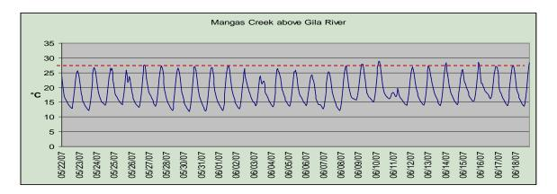
**Figure 2.** Example of assessable dataset for non-support determination (applicable segment-specific maximum criterion of 28°C is exceeded on more than one day in this limited duration dataset)
