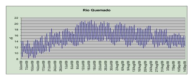
**Figure 1.** Example of assessable dataset for full support determination (adequate duration and includes summer season maximum temperature less than applicable maximum criterion of 23°C)
