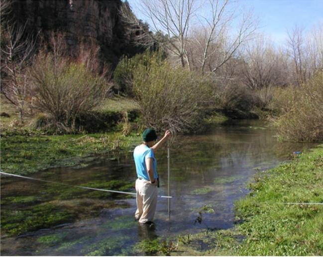
Fig. 2–21. Current meters are best used in higher volume streams.
