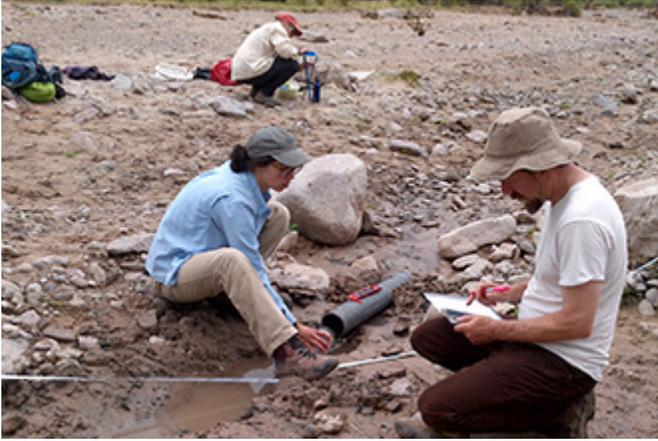
Fig. 2-17. Crews measure flow by creating a dam out of soil to direct the flow through a pipe.
