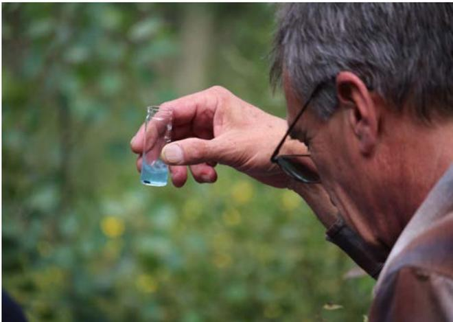
Fig. 2–23. Test kits are available to accurately measure field water quality characteristics, such as alkalinity. These require no calibration, are relatively inexpensive, and provide a useful backup system for electronic units.
