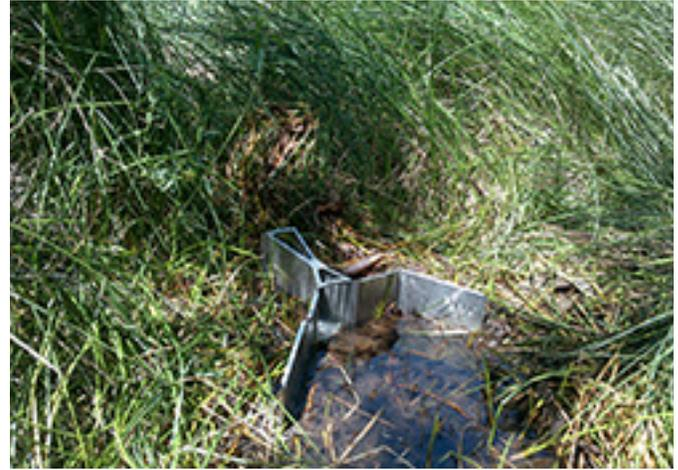
Fig. 2-20. Cutthroat flumes are useful for more challenging settings. Although “portable”, they are heavy and awkward for use in remote sites. This flume was used to measure flow at a helocrene in New Mexico.
