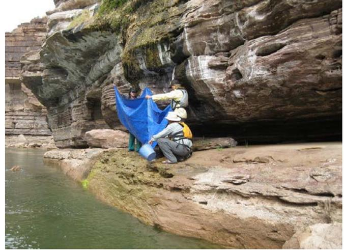
Fig. 2-18. Surveyors occasionally must improvise in order to measure flow. In this case the crew used a tarp to collect dripping water at a hanging garden spring on the bank of the Colorado River in Grand Canyon, Arizona.
