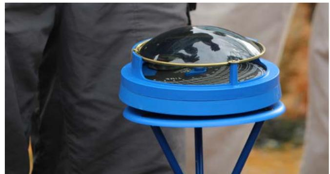
Fig. 2-4. Solar Pathfinder is used to measure the photosynthetically active radiation at a springs ecosystem.
