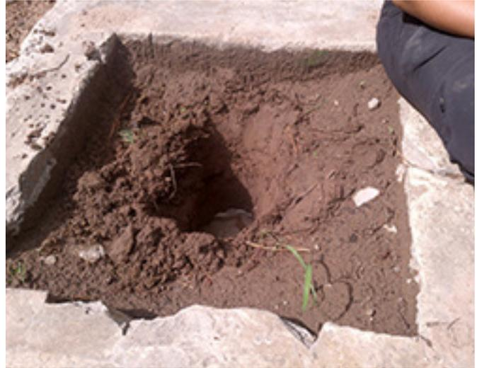
Fig. 2–16. In this case, surveyors dug a hole and measured time to refill in order to measure flow.
