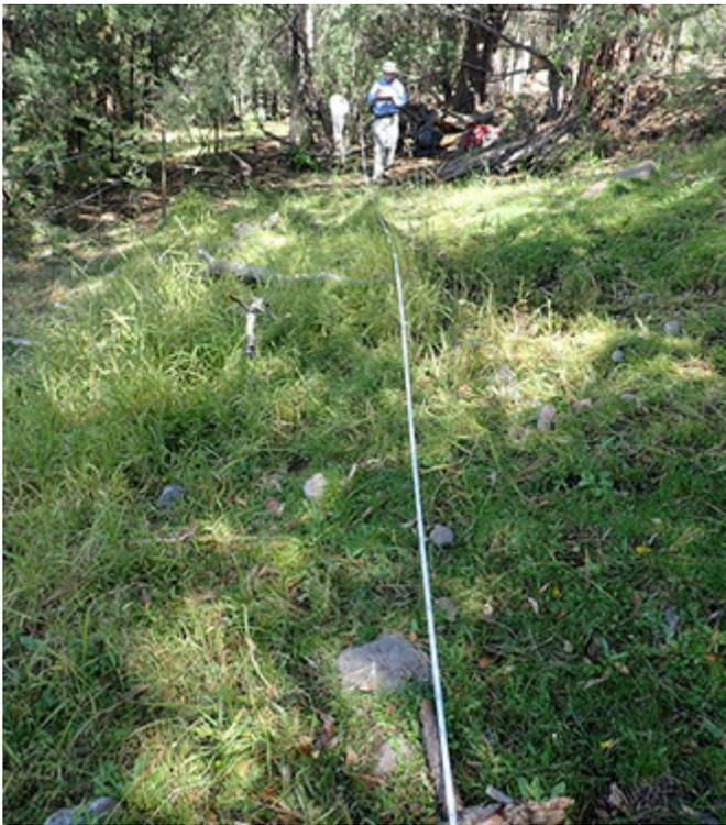
Fig. 2-5. The survey crew should stretch a metric tape along the long axis of the site, and perpendicularly. Photo credit Emile Sawyer.
