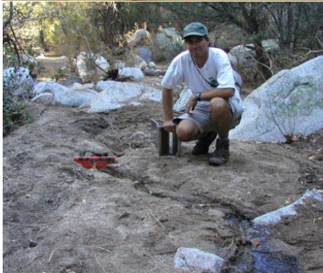
Fig. 2-19. Hydrologists use a V-notch weir plate to measure low volume flows in soft substrate.
