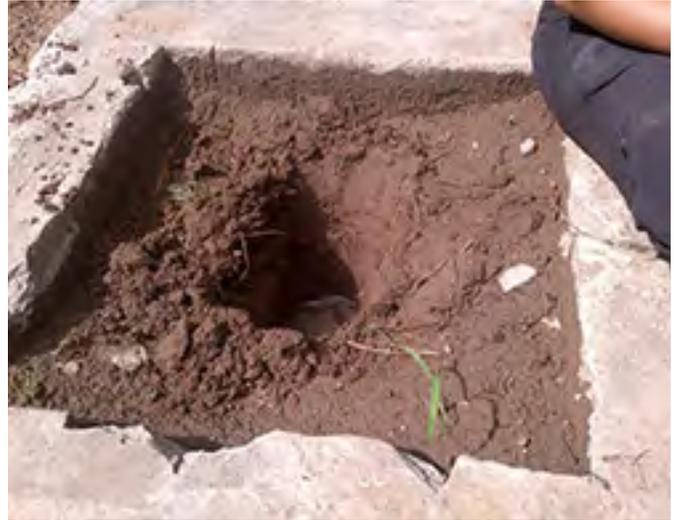
Fig. 5-17. In this case, surveyors dug a hole and measured time to refill in order to measure flow.
