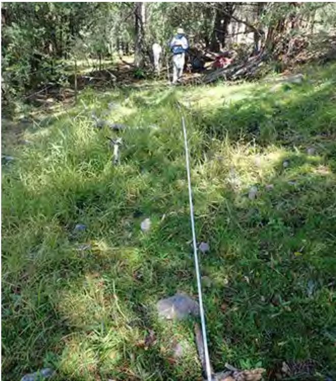
Fig. 5–6. The survey crew should stretch a metric tape along the long axis of the site, and perpendicularly. Photo credit Emile Sawyer.
