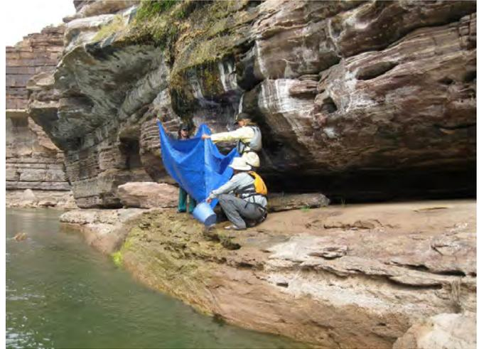
Fig. 5-19. Surveyors occasionally must improvise in order to measure flow. In this case the crew used a tarp to collect dripping water at a hanging garden spring on the bank of the Colorado River in Grand Canyon, Arizona.
