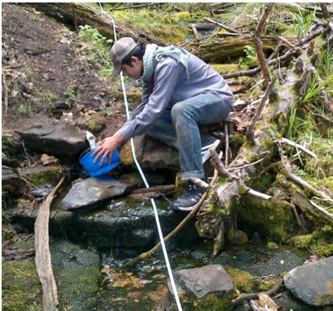
Fig. 5–2. Most springs inventory protocols include measurement of discharge.
