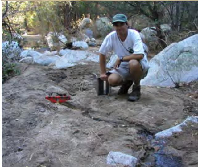
Fig. 5-20. Hydrologists use a V-notch weir plate to measure low volume flows in soft substrate.
