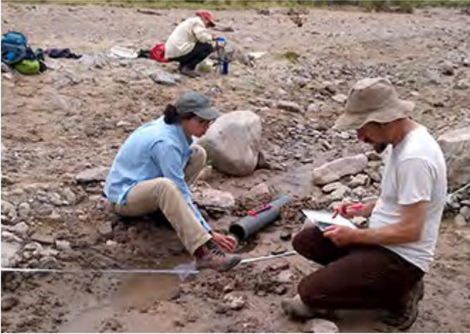
Fig. 5-18. Crews measure flow by creating a dam out of soil to direct the flow through a pipe.
