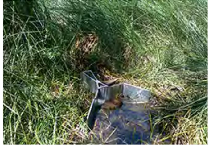
Fig. 5-21. Cutthroat flumes are useful for more challenging settings. Although "portable", they are heavy and awkward for use in remote sites. This flume was used to measure flow at a helocrene in New Mexico.
