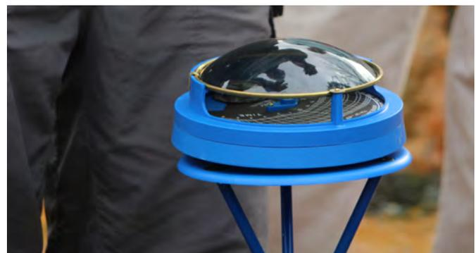
Fig. 5-5. Solar Pathfinder is used to measure the photosynthetically active radiation at a springs ecosystem.
