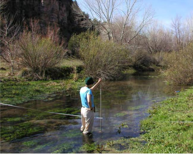
Fig. 5–22. Current meters are best used in higher volume streams.
