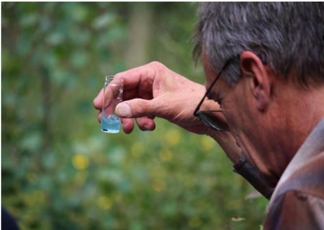
Fig. 5–24. Test kits are available to accurately measure field water quality characteristics, such as alkalinity. These require no calibration, are relatively inexpensive, and provide a useful backup system for electronic units.
