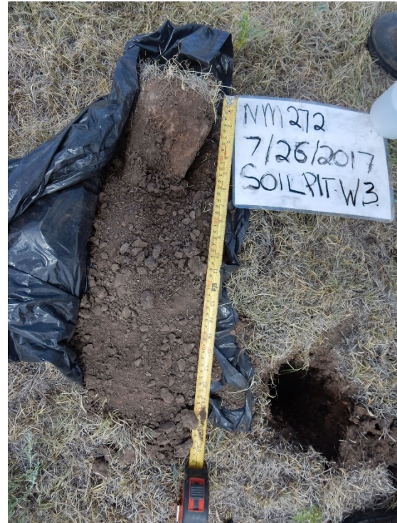
Figure 8. A documentary photograph of the soil sample is recommended. The top of the tape measure is the top of the core.
