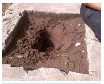
Fig. 2–16. In this case, surveyors dug a hole and measured time to refill in order to measure flow.
