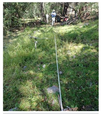
Fig. 2–5. The survey crew should stretch a metric tape along the long axis of the site, and perpendicularly. Photo credit Emile Sawyer.
