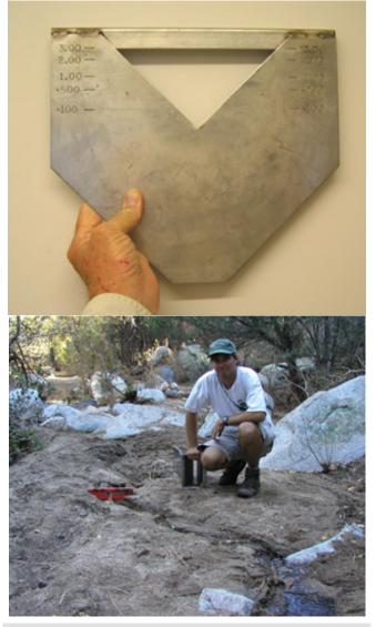
Fig. 2–19. Hydrologists use a V-notch weir plate to measure low volume flows in soft substrate.
