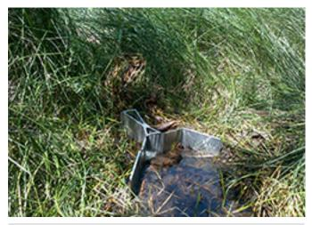
Fig. 2–20. Cutthroat flumes are useful for more challenging settings. Although "portable", they are heavy and awkward for use in remote sites. This flume was used to measure flow at a helocrene in New Mexico.
