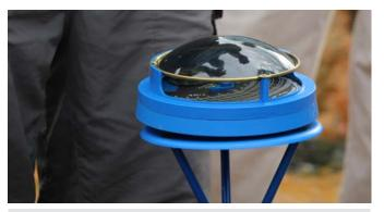
Fig. 2–4. Solar Pathfinder is used to measure the photosynthetically active radiation at a springs ecosystem.
