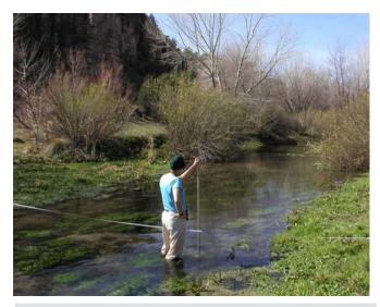
Fig. 2–21. Current meters are best used in higher volume streams.
