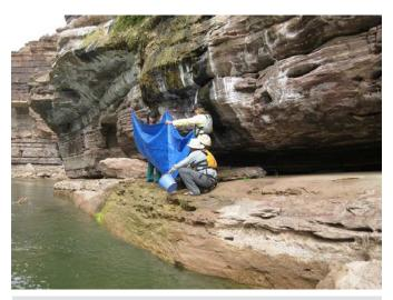
Fig. 2–18. Surveyors occasionally must improvise in order to measure flow. In this case the crew used a tarp to collect dripping water at a hanging garden spring on the bank of the Colorado River in Grand Canyon, Arizona.
