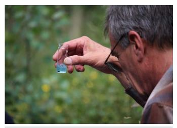
Fig. 2–23. Test kits are available to accurately measure field water quality characteristics, such as alkalinity. These require no calibration, are relatively inexpensive, and provide a useful backup system for electronic units.
