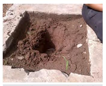
Fig. 5–17. In this case, surveyors dug a hole and measured time to refill in order to measure flow.
