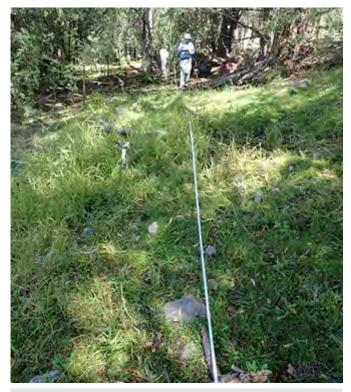
Fig. 5–6. The survey crew should stretch a metric tape along the long axis of the site, and perpendicularly. Photo credit Emile Sawyer.
