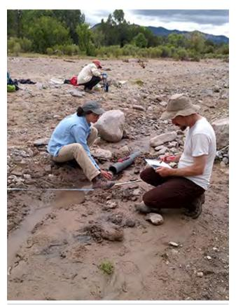
Fig. 4–2. Flow measurements at rheocrene springs can be strongly affected by runoff.
