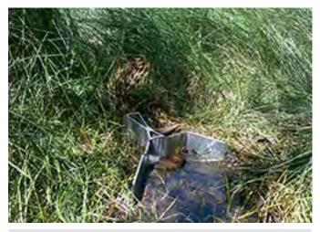
Fig. 5–21. Cutthroat flumes are useful for more challenging settings. Although "portable", they are heavy and awkward for use in remote sites. This flume was used to measure flow at a helocrene in New Mexico.
