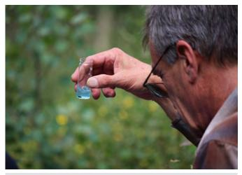
Fig. 5–24. Test kits are available to accurately measure field water quality characteristics, such as alkalinity. These require no calibration, are relatively inexpensive, and provide a useful backup system for electronic units.
