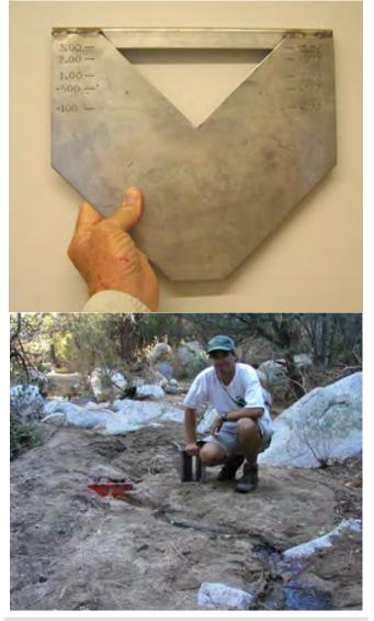
Fig. 5–20. Hydrologists use a V-notch weir plate to measure low volume flows in soft substrate.
