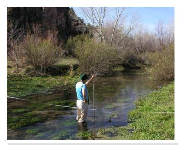
Fig. 5–22. Current meters are best used in higher volume streams.
