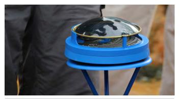
Fig. 5–5. Solar Pathfinder is used to measure the photosynthetically active radiation at a springs ecosystem.
