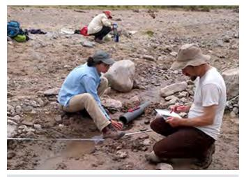
Fig. 5–18. Crews measure flow by creating a dam out of soil to direct the flow through a pipe.
