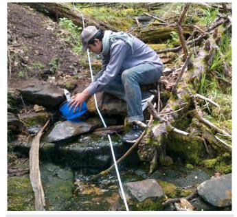
Fig. 5–2. Most springs inventory protocols include measurement of discharge.
