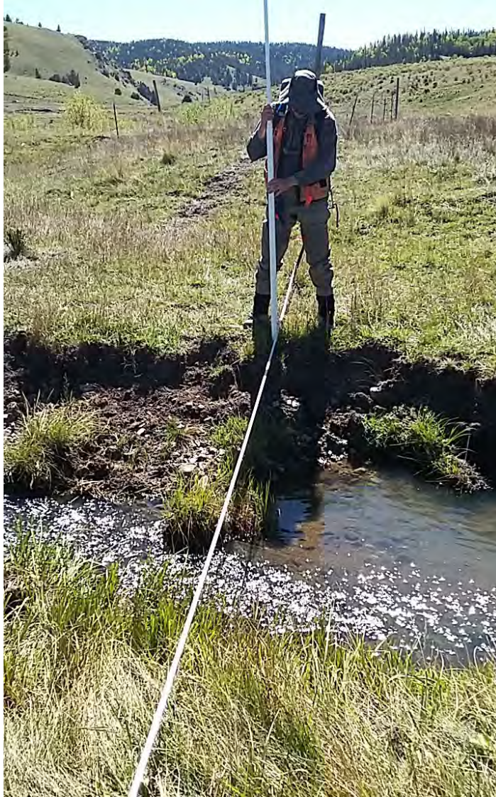
Figure 1: SWQB staff conducting long-term geomorphology monitoring on Comanche Creek, in support of a watershed-based planning project there. September 2017 photograph by Alan Klatt.
