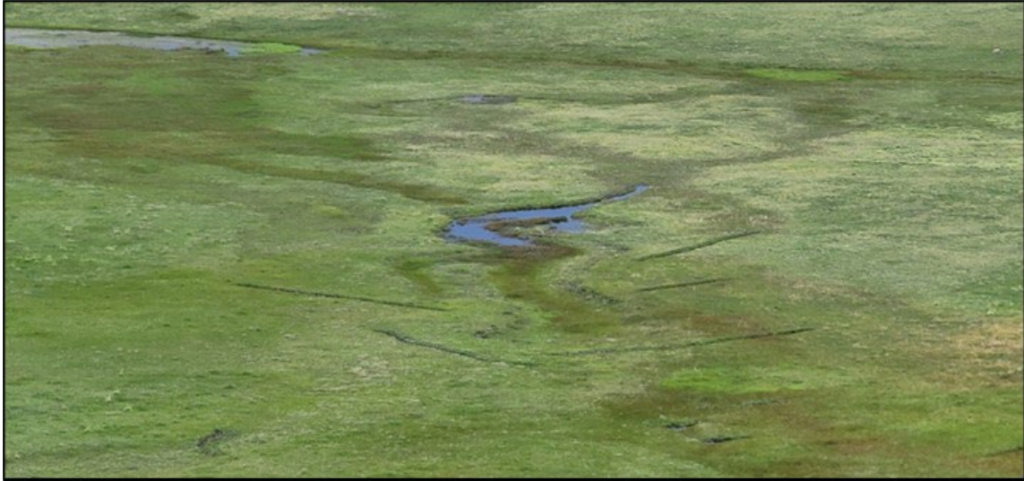
Figure 1 Plug and Pond Restoration Structures on the East Fork. The very top of the gully formation can be seen here at the bottom of the photo. Darker lines are contour swales diverting water flow away from the headcut and spreading water to surrounding areas,
