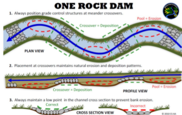
One Rock Dam Schematic. Figure from Sponholtz and Anderson (2013)
