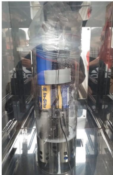
18. Next, record the temperature of the water displayed on the NIST certified thermometer at the same time interval set for sondes(s) to record data points on the **Temperature Accuracy Verification Spreadsheet**. Ensure at least 3 temperature measurements are recorded at least 5 minutes apart between 35-40 °C.
