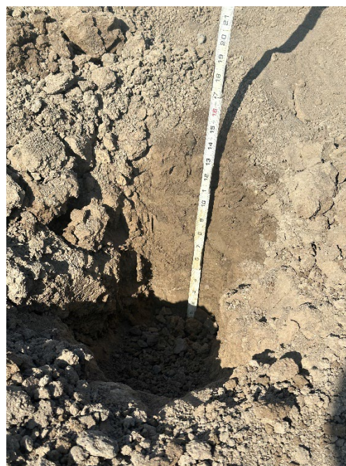
FIGURE 54 CLAY SOILS WITH DEEP CRACKS, PLAYA 950.
