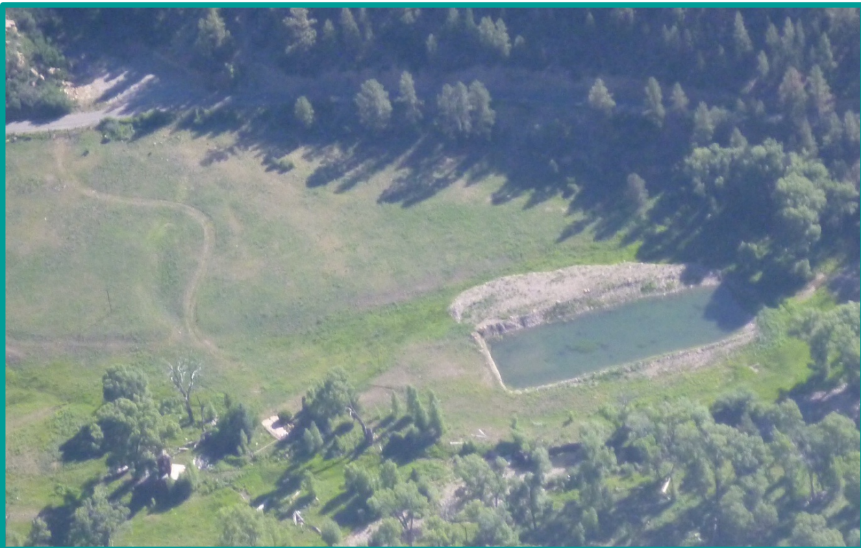
Figure 14. Aerial photograph of a man-made pond that could be restored by modifying the bank shape and planting riparian vegetation (downstream of G8).
