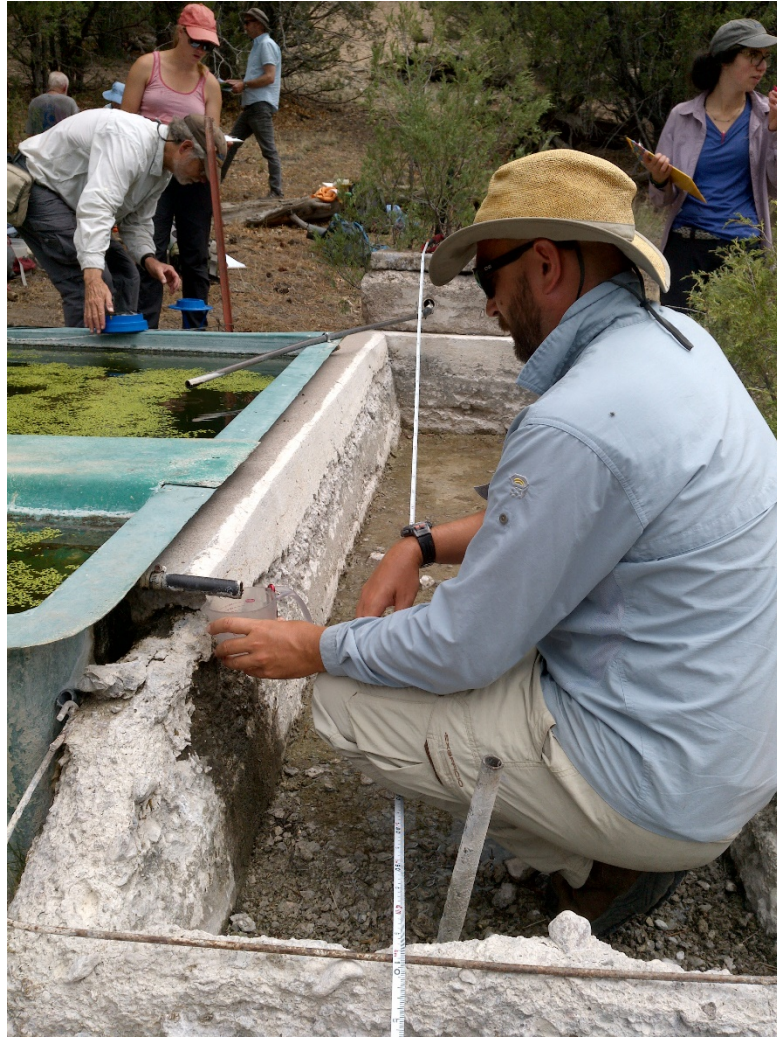
Figure 6. Ed Schenk from MNA-SSI measuring spring flow at a developed spring near Quemado, NM
