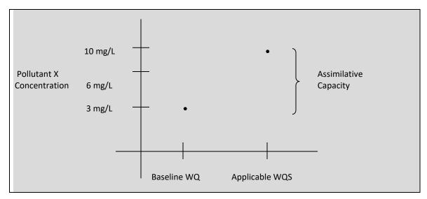
Figure 5-1. Simplified Representation of Assimilative Capacity
