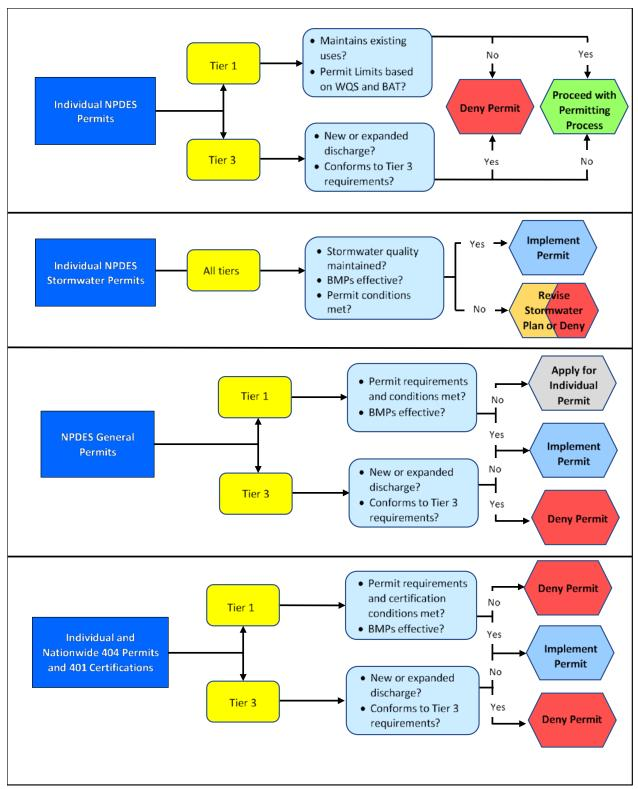
Figure 3-2. Antidegradation Review Requirements by Permit Type
