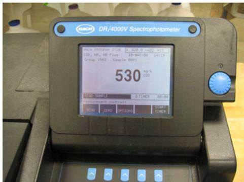
6. Using a kimwipe®, wipe off the outside of the sample. Insert the sample into the sample holder with the Hach name facing forward. Close the cover and press the READ button. Record the display value on the data sheet.
