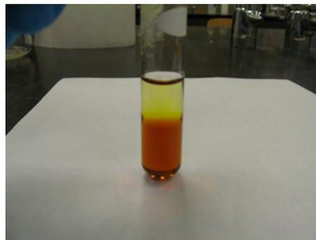
The heat will be provided by the digestion reactor which is set at  $150^{\circ}C$ . The sample is refluxed (digested) for 2 hours. During the 2 hours, the organics are oxidized by the acid, potassium dichromate and catalyst.
