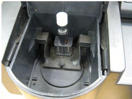
Figure: Insert tube into cell holder
