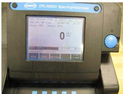
Figure: Zero the spectrophotometer using a reagent blank.
