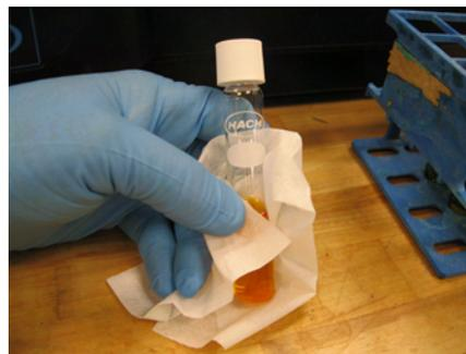
Figure: Wipe with kimwipe® to remove fingerprints, dirt.
