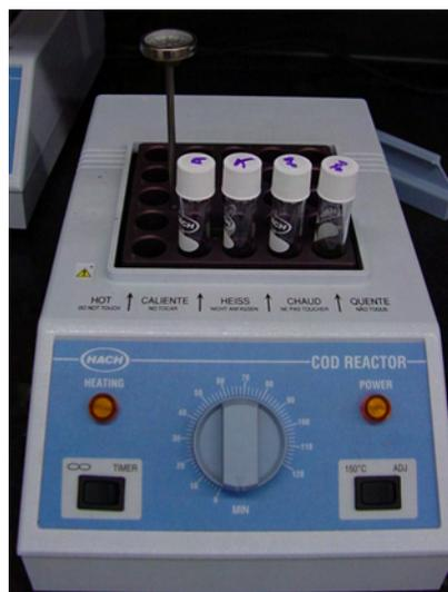
The catalyst is silver. However, silver must be soluble and will precipitate if chlorides are present in the sample. To prevent silver precipitation, mercury has been added to the reagents in the tube. The mercury will remove the chloride interference.
