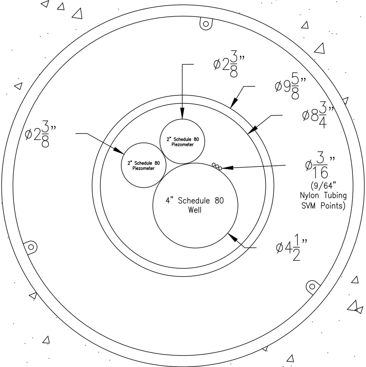
Distance Between Casing and Borehole is approximately 0.8"
