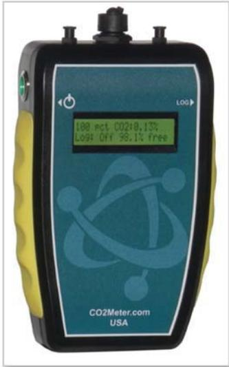
This portable battery-powered CO2Meter, Inc. meter is designed to measure carbon dioxide (CO2) in real-time in inaccessible areas for applications like fermentation vats & barrels, biological incubators, and CO2 leak detection. Its internal memory allows the user to record CO2 concentration level data over time.
