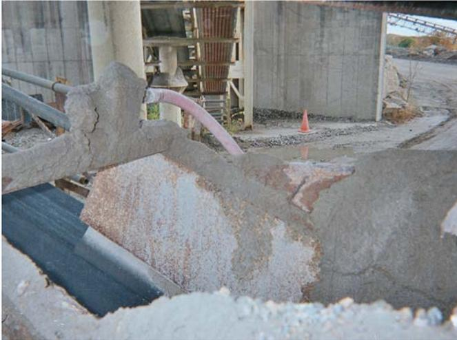
*Deposition on spray bars is a common cause of nozzle pluggage.*
