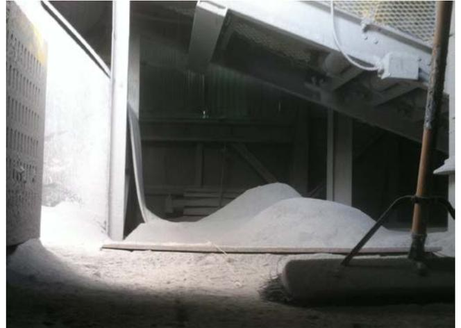
*Workers get their greatest exposure to silica-containing dust when they have to clean up spillage resulting from inadequate enclosure.*
