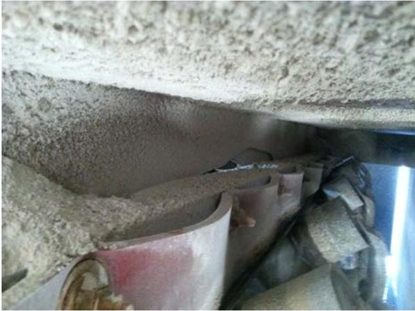
*Worn skirts and leaks in chutes allow dust and spillage to escape*
