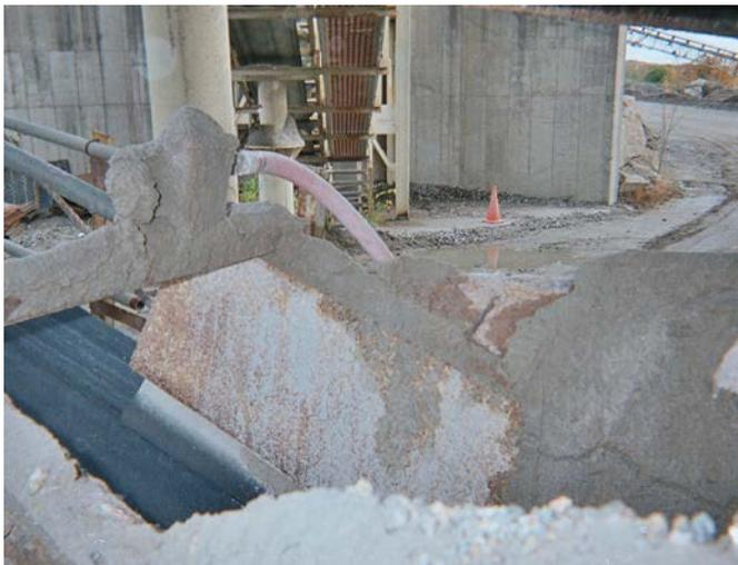
*Deposition on spray bars is a common cause of nozzle pluggage.*
