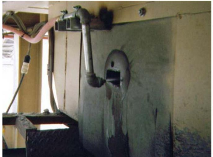
*Protect nozzles from deposition that can plug them up by installing a dust curtain that protects them from the "blowback" of mist and wet fines.*
