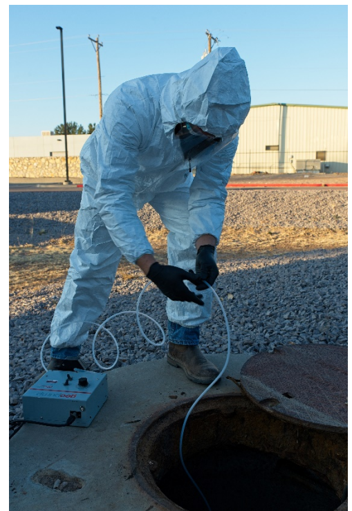
A sampler gathers a wastewater at a collection point.
