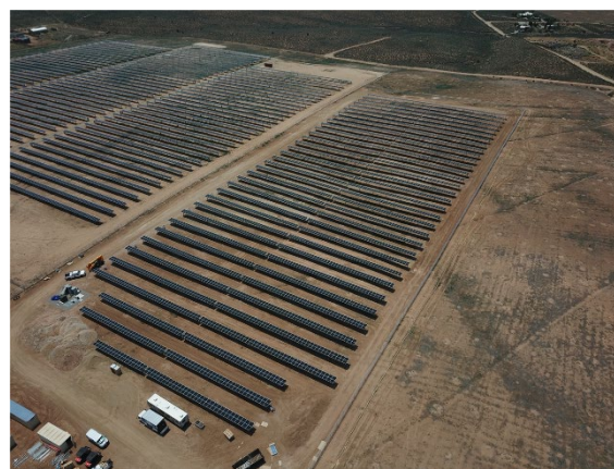
Photo 5: Aerial photo of the new Town of Taos 1-MW and 80-kW solar array. The system will generate solar energy and provide electricity directly to the WWTP. This photo is courtesy of Affordable Solar.
