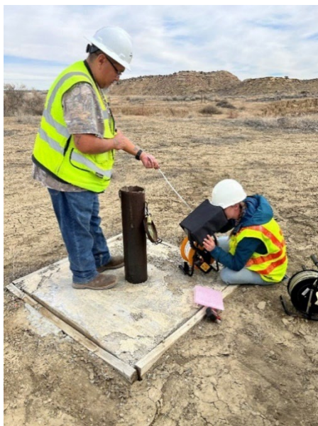
Photo 1: Avery Young of the Ground Water Quality Bureau views the progress of a well camera as it descends the well casing to determine if well construction was properly completed and to check for any compromised sections. She is aided by a local utility operator.
