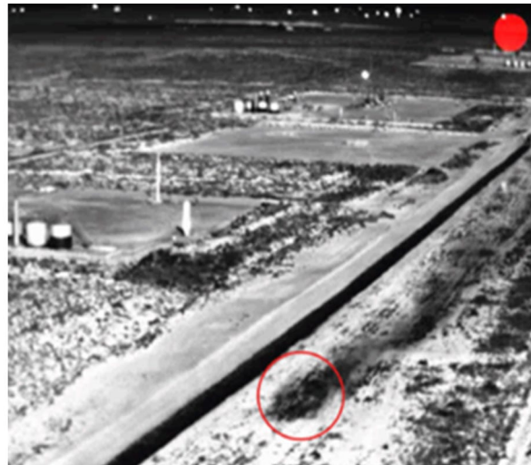
Thermal imaging of pipeline release.
