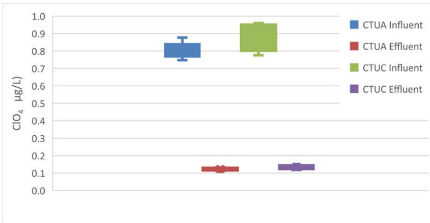
Figure 5. IX Treatment System 2016 Paired Perchlorate Influent/Effluent Results.
