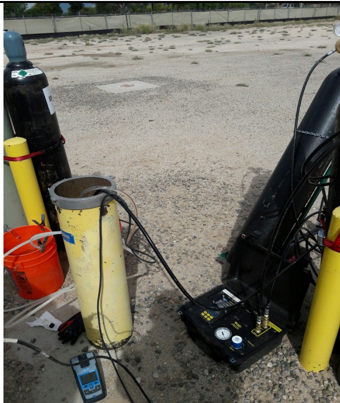
Description: Groundwater sampling setup with high pressure controller for bladder pump.
