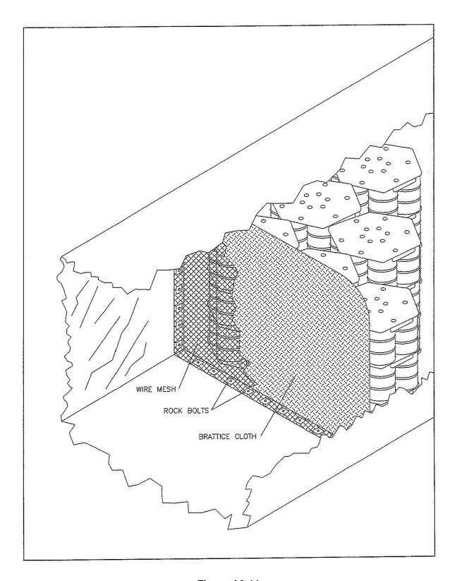
Figure A2-11 Typical Room Barricade
