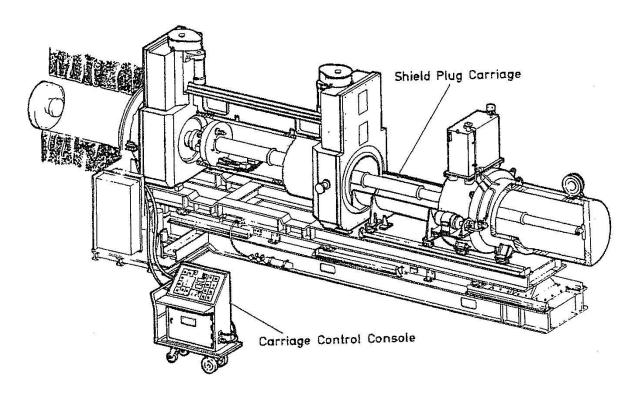
Figure A2-18 Installing Shield Plug
