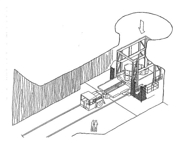
Figure A2-6 Waste Transfer Cage to Transporter
