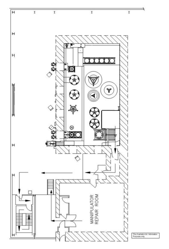
Figure D-6b RH Bay Hot Cell Evacuation Route
