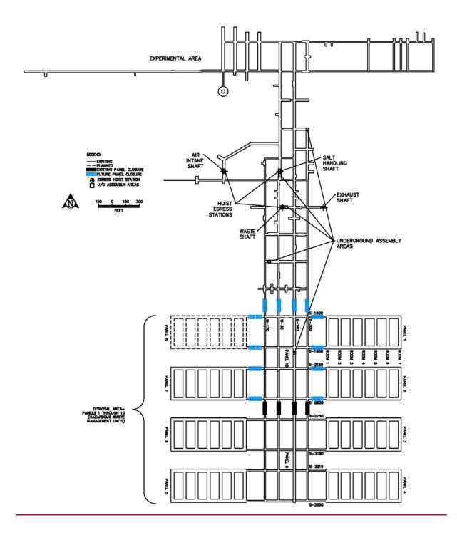
Figure D-7 Designated Underground Assembly Areas
