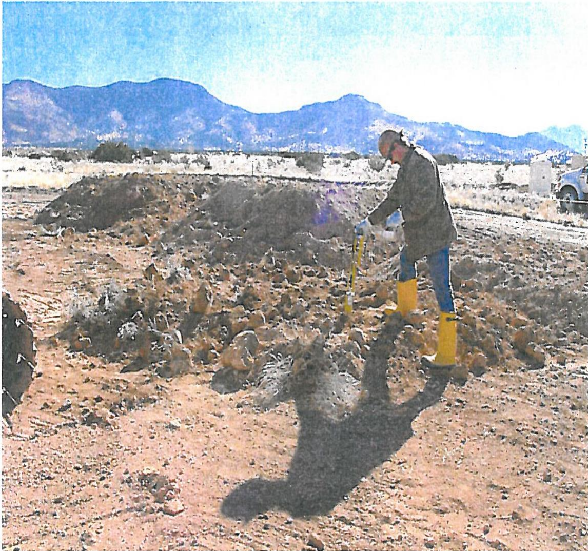
Figure 15. Radiological Screening of Soil during Excavation of the SWMU 68 Burn Pan
