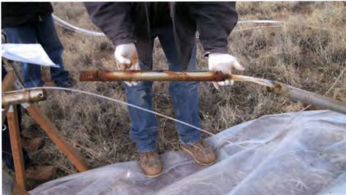
Figure 10. Photograph of the stainless steel Bennett™ sampling pump after removal from MWL-MW4 on December 16, 2014 showing substantial corrosion
