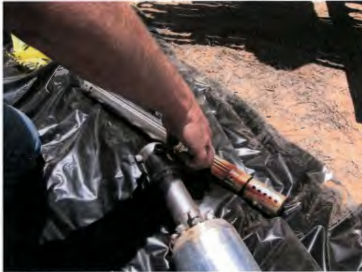
Figure 5. May 2009 Photograph of the MWL-MW4 Sampling Pump and Inflatable Packer
