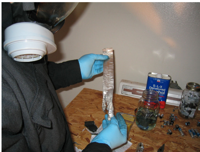
Figure 1. Obtaining lithium metal from photographic batteries.
