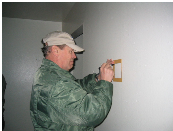
Figure 2. Using a 100 cm 2 template to mark a wipe sampling location at the cook site.
