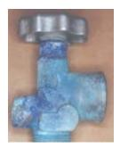
As observed in the illustrations, a blue-green stain on any brass valve is evidence that it may have been in contact with anhydro pungent odor of ammonia on or near the cylinder is also an indi that a propane cylinder contains or has contained anhydrous ar extreme caution and restrict access to the area.
