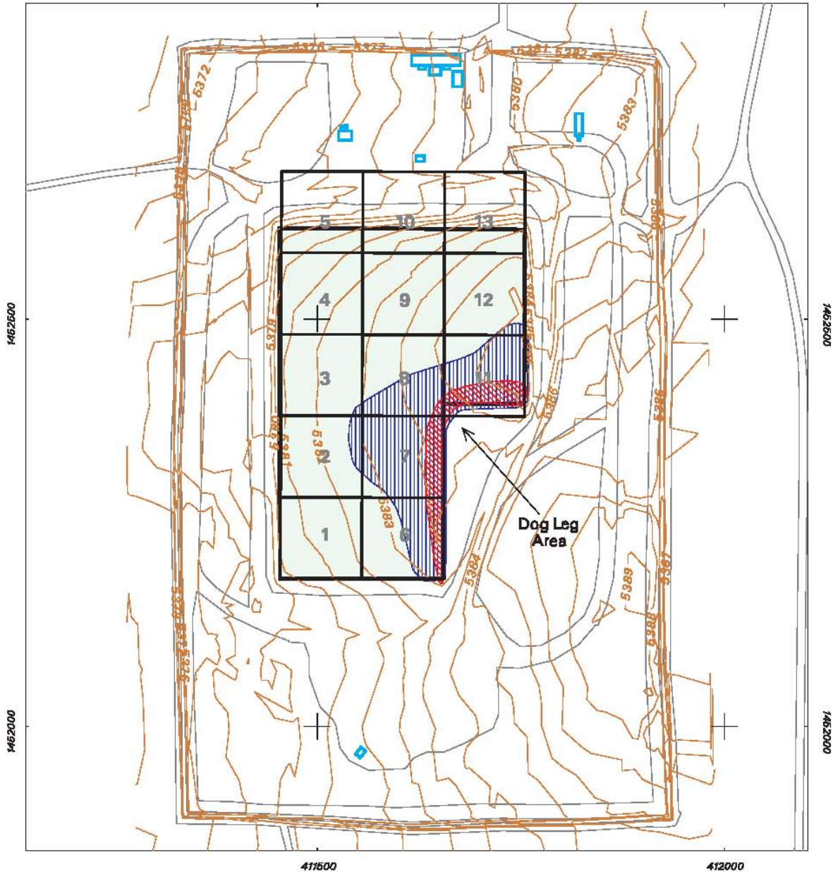
Figure 3 Mixed Waste Landfill Cover Grid Blocks and Locations of Native Soil Layer Wedge Lifts 1 & 2
