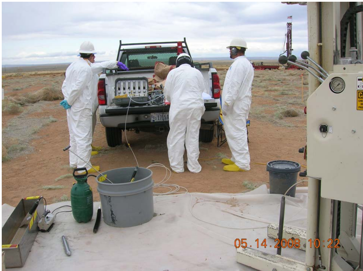
Figure 4-4 Collecting a Soil-Vapor VOC Sample at the Mixed Waste Landfill, May 14, 2008 (view to the west).
