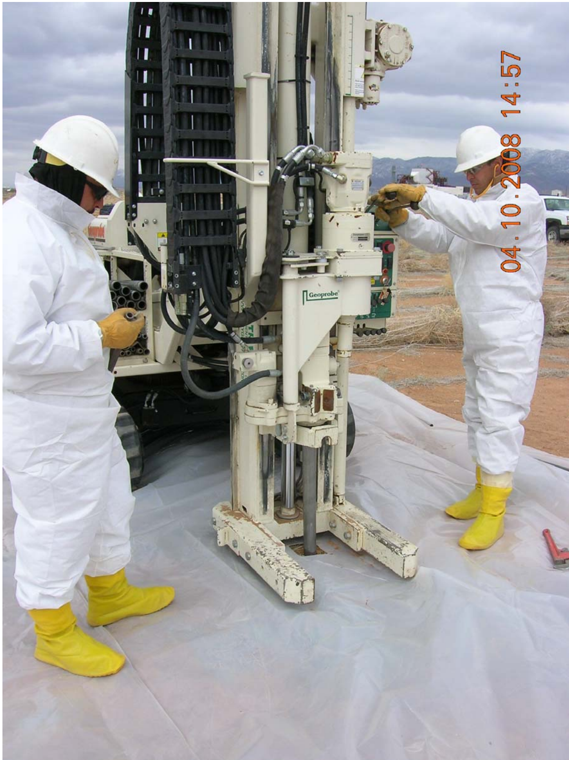
Figure 4-2 Collecting Tritium Soil Samples with the Geoprobe® at the Mixed Waste Landfill, April 10, 2008 (view to the northeast).
