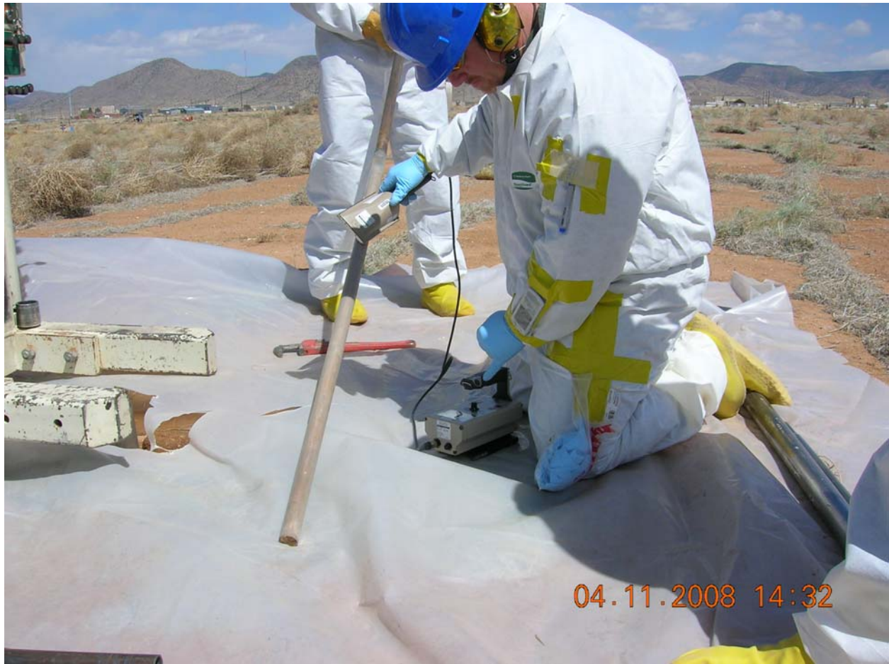
Figure 4-3 Scanning a Soil-Filled Geoprobe® Butyl Acetate Sleeve for Radiological Contamination at the Mixed Waste Landfill, April 11, 2008 (view to the east).
