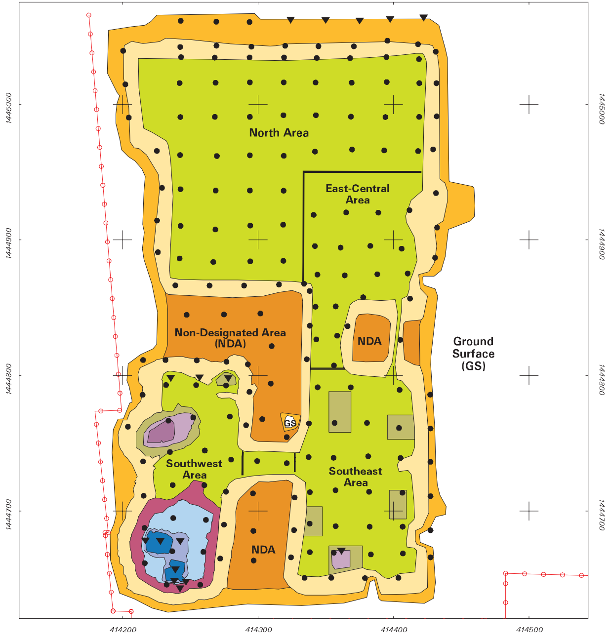
Figure 5 Extent of LE VCM Excavation and Final Verification Soil Sampling Grid Locations
