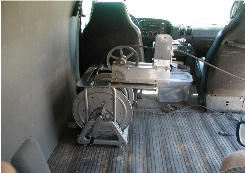
Cable reel used to lower CPN probe into the VZ access tubes
