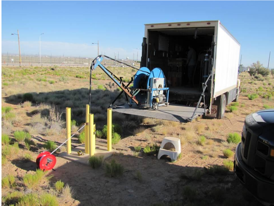
Figure 3.3-1 Groundwater Sampling Truck with Bennett™ Pump and Solinst Water Level Meter (red reel in left foreground) Deployed in the Monitoring Well
