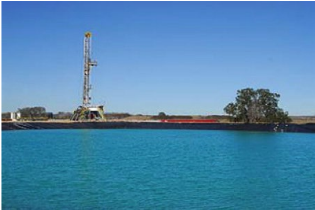
Figure 2-19: A Pioneer Drilling Rig Behind the Lined Containment Berm of a Water Storage Pond
