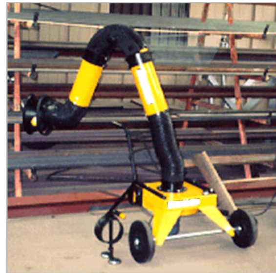
Local exhaust ventilation
