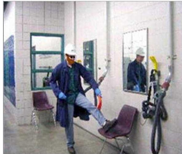
Vacuum to remove lead from clothing
