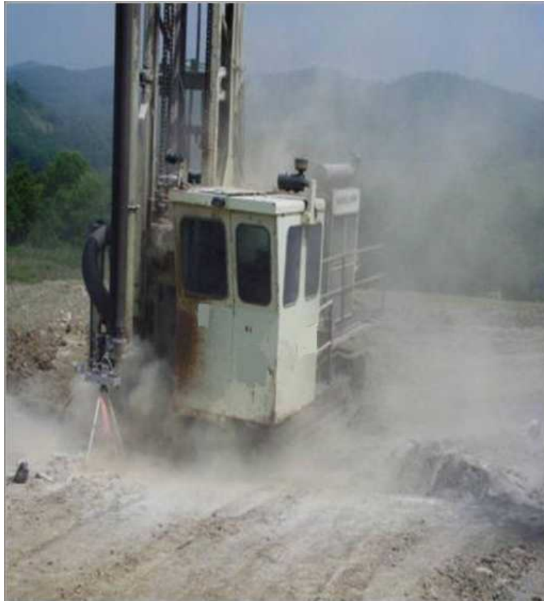
No engineering controls
