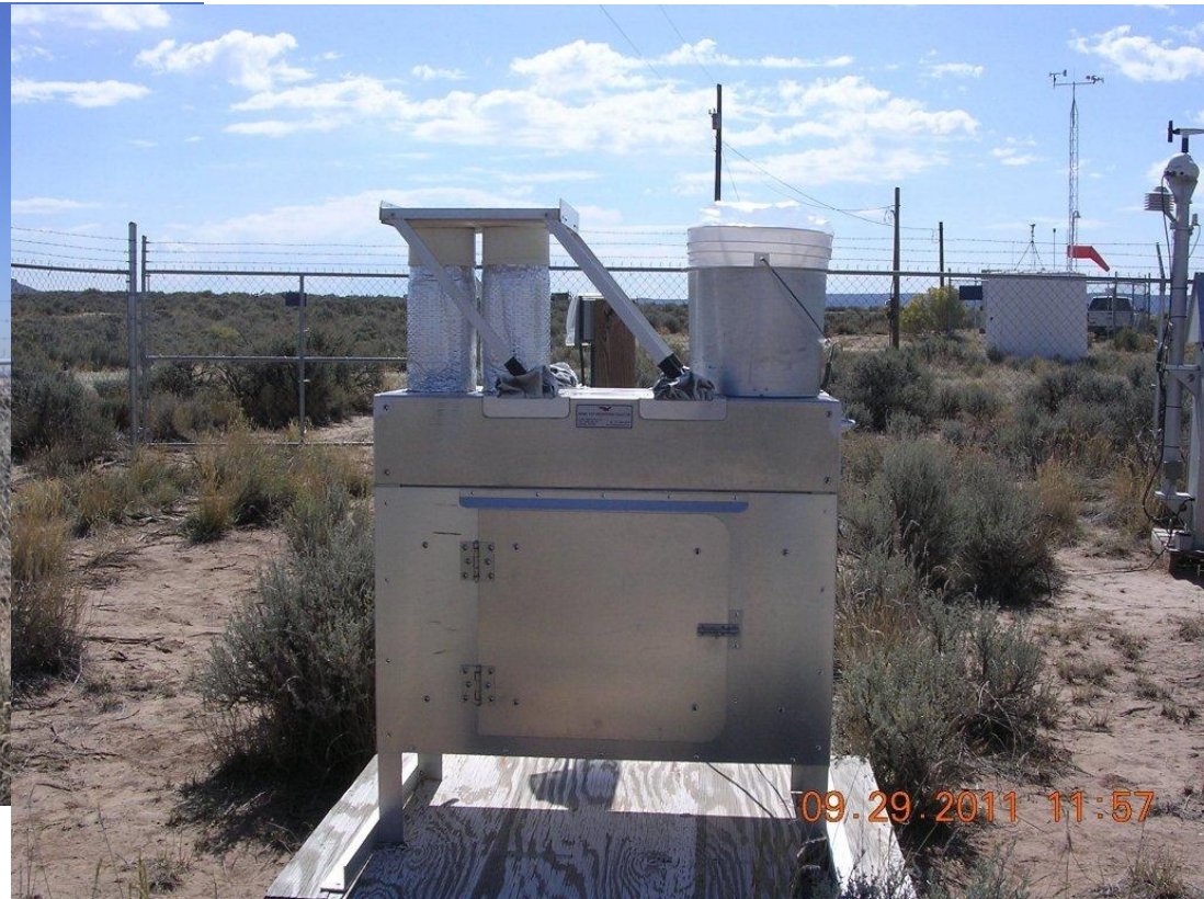
Navajo Lake Site, NM Monitor type: Wet Deposition Mercury Study duration: recently discontinued
