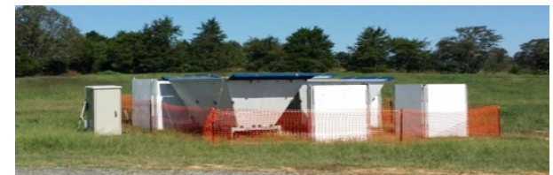
NOAA 915 MHz Wind Profiling Radar at 2 sites: Navajo Lake and near Farmington (photo from another campaign in AR)
