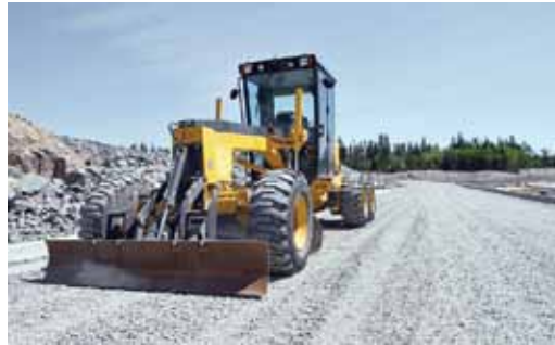
Figure 13: A road grader with front dozer blade is used to spread gravel over soil. Gravel is an expensive but effective dust suppressant for areas heavily used by motor vehicles.
