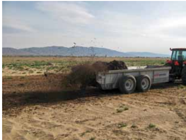
Figure 10: A fertilizer spreader can be used to cover unstable soil with a uniform 2-3 inch layer of wood chips.
