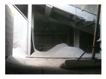
Workers get their greatest exposure to silicacontaining dust when they have to clean up spillage resulting from inadequate enclosure.
